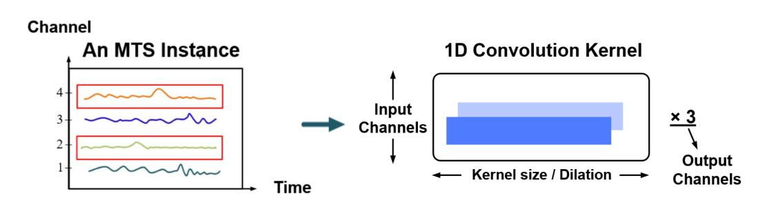
Input specific channels of a multivariate time series (MTS) instance for the designed 1D convolutional kernels
