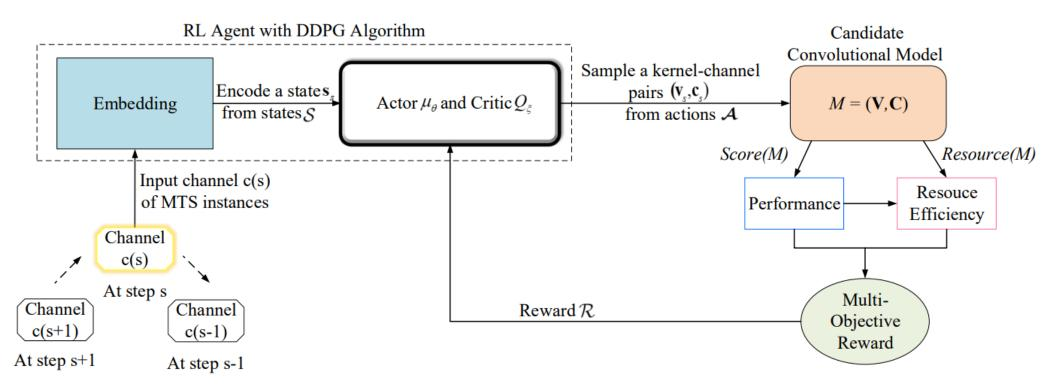
Automatically generate 1D convolutional kernels to transform specific channels of input time series data into discriminative representations
